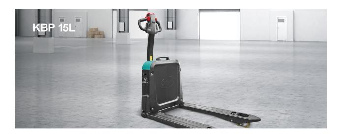
The KBP 15L, with a load capacity of 1.500 kg and its compact size of only 400 mm to face of forks, is the Baoli pallet truck for any medium duty application in warehouses, logistics and industry.
