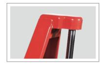
2 Chassis with robust upper steering bearing for less friction and steering force.
